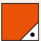
The orange swatch with the little triangle and dot in the bottom right corner (see far left) means that the colour is a spot colour. All the other colours in the panel are 4 colour process.
